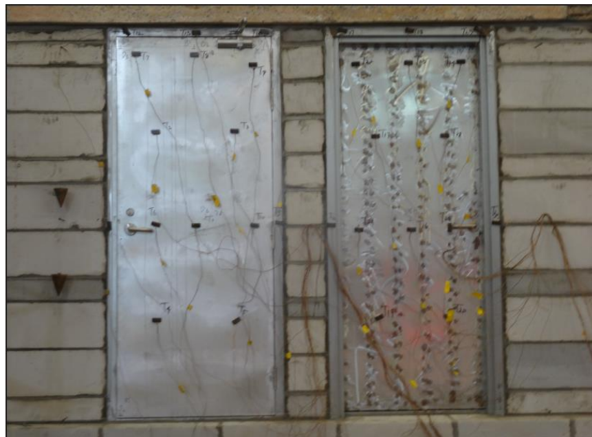
Fig. 2 Unexposed Side Prior to the Fire Test
