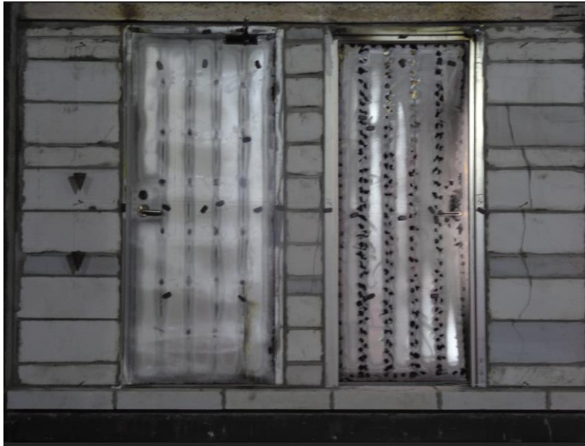
Fig. 5 Unexposed Side after 260 Minutes
